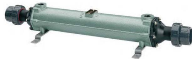
The CN S Series heat exchangers have Cupro Nickel Titanium or Stainless Steel tubes encased in cast steel with composite end covers that have solvent weld connections that fit directly into pool pipework. These series are made specifically for Solar, Geothermal and Heat Pump applications and are ideal for salt water pools and spas.
